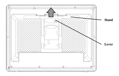
(2) Slide the stand to the desired angle, and release the lever.
