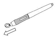
(2) Insert a new pen tip into the stylus pen.
