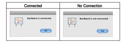
If they are connected properly, the "StarBoard is connected" message appears. If the indication does not change even though you have checked the connection, there is likely to be some problem. For details, see "3. Appendix Troubleshooting" on page 3-1 in this user's guide.
