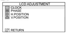
CLOCK : Used to adjust screen size. (0-100)
